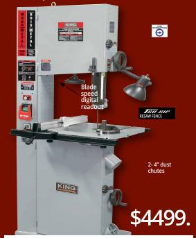
Comes with: a 1/2" x 6 TPI wood cutting blade, 1/2" x 10 TPI metal cutting blade, laser guide, work lamp, miter gauge and a precision "TRU-RIP" aluminum rip fence with resaw guide
